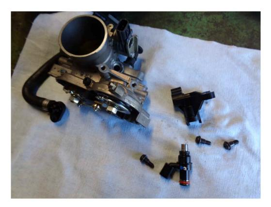
As an aside, the link to my 'make your own' Throttle Position Sensor tool: http://www.acproducts.co.uk/docs/Husqvarna\_KTM\_TPS\_tool.pdf Setting the TPS is critical and rarely correct from the factory on a new machine.
