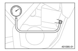
Position the special tool. Mount and tighten the banjo bolt.
